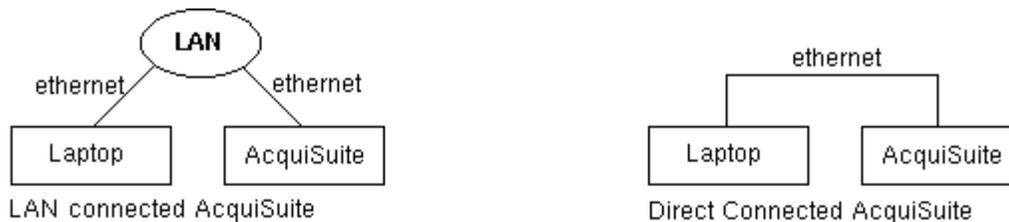
The remainder of this section will assume the installer has brought a laptop to the site, and will connect the laptop to the building LAN, or directly to the AcquiSuite. Attach the laptop to the AcquiSuite or LAN as shown in figure 6, Ethernet hookup.
